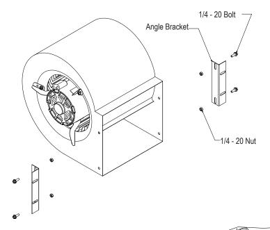
2. Attach blower to the left and right mounting brackets.
